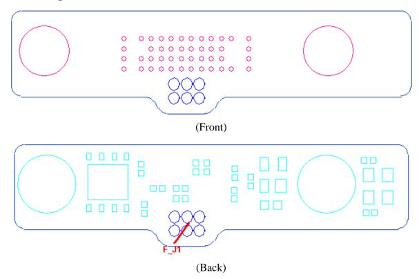
Figure B-6 Finger Printer Board layout (front/back)
